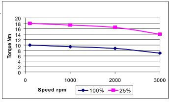
Data• were measured on an HDD14J-Pa series motor mounted on a vertical 450 x 375 x 30 mm steel plate in free air, with a winding temperature rise of 90°C and driven by a commercially available inverter.
