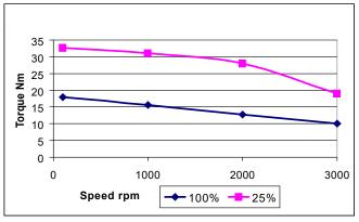
Data• were measured on an HDD14N-Pa series motor mounted on a vertical 450 x 375 x 30 mm steel plate in free air, with a winding temperature rise of 90°C and driven by acommercially available inverter.
